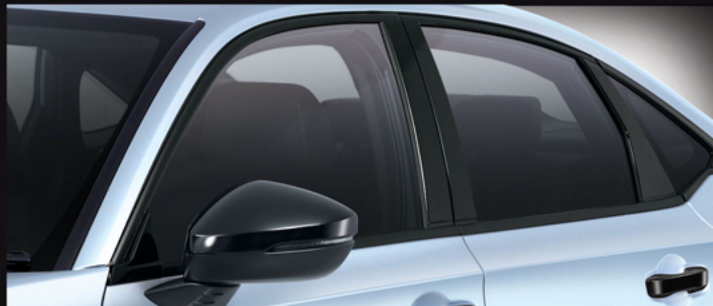
BLACK PAINTED DOOR MIRRORS: Black painted door mirrors that are retracted automatically as car doors are locked/unlocked.
