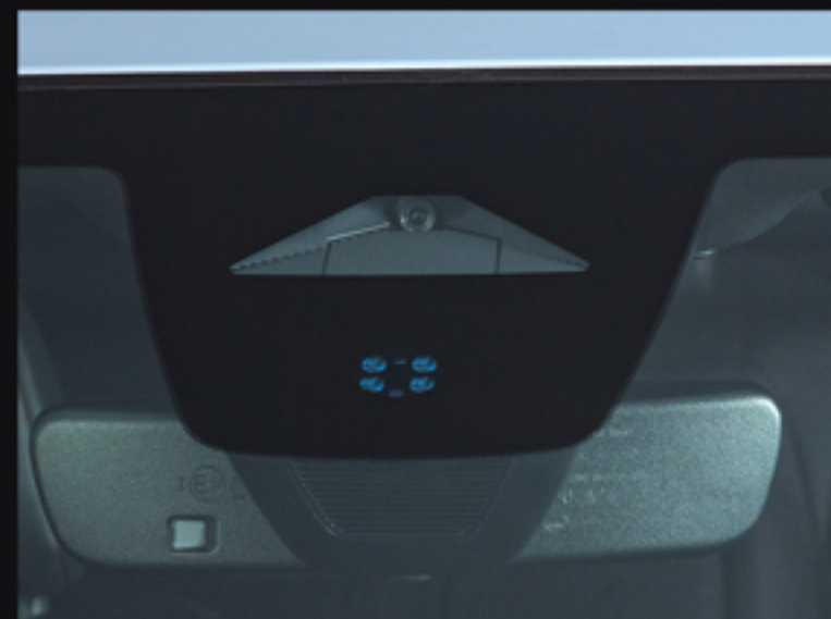
RAIN SENSOR: Automatically activate wipers.
